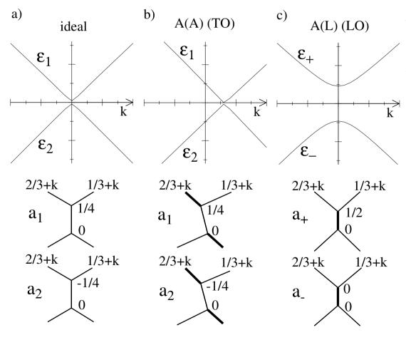
first principles band structure in the vicinity of  $k_F$  for the (12,0) zigzag nanotube in a) the equilibrium positions, b) for a distortion compatible with the A(T) mode, and c) for a distortion compatible with an A(L) mode below each band-structure diagram, the phase  $\phi$  of the eigenstates  $a_i$  (corresponding to the band with energy  $\varepsilon_i$ ) are shown for states in the vicinity of  $k_F$
