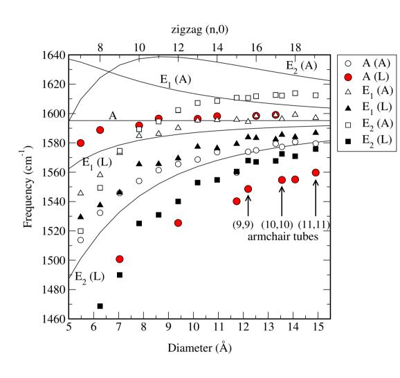
phonon frequencies of (n,0) zigzag and (n,n) armchair tubes and in the G-band calculated by *ab initio* density functional theory (symbols) and zone folding (lines, using force constants calculated by same density functional approach)
