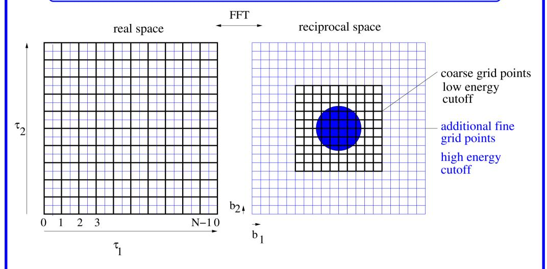
data transfer occurs only in reciprocal space, grids are not necessarily "aligned" evaluation of the potentials (XC) is also done on the fine grid, which often saves you in GGA
