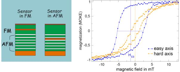
Left: Exchange bias system with an antiferromagnetically coupled superlattice acting as AFM. <sup>57</sup>Fe sensor layers are placed in the FM and AFM.
